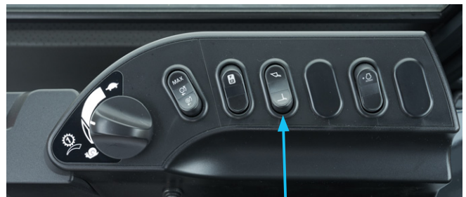
Attachment selector switch
