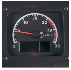
• **Speedometer/Tachometer Module.** Monitors three systems: engine speed, ground speed and gear indicator.
