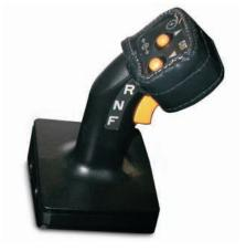
STIC™ Steering Control. STIC™ combines directional selection, gear selection and steering into a single lever for maximum responsiveness. Simple side-to-side motion turns machine right or left. Transmission shifting (forward/neutral/reverse) is controlled using a three position rocker switch. The thumb operated upshift and downshift buttons control manual shifting.
