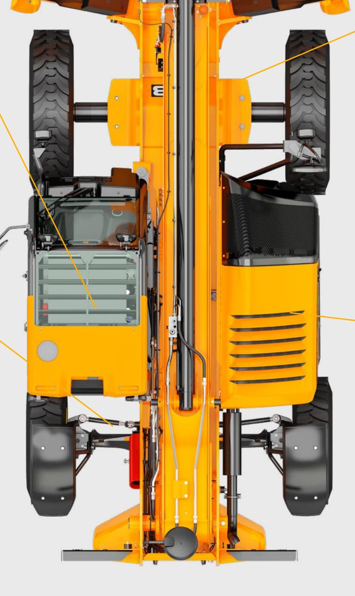
JCB chassis are designed using a 20/25 mm side plates to aid stability and durability when operating in the most demanding environments.
