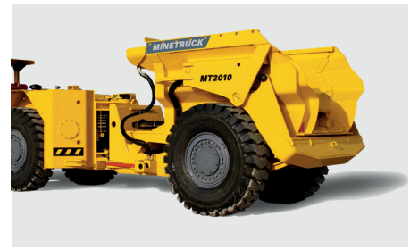
Optional Teletram dump box to release materials horizontally in areas with a low back height.
