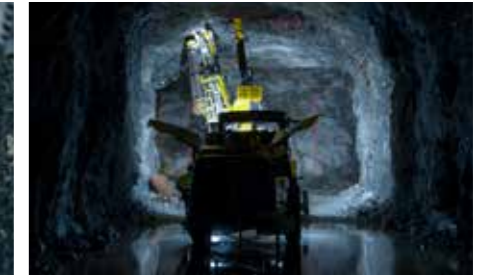
The Boltec M series machines share a common four wheel drive articulated carrier design with their Simba M/E and Boomer M/E stablemates.
