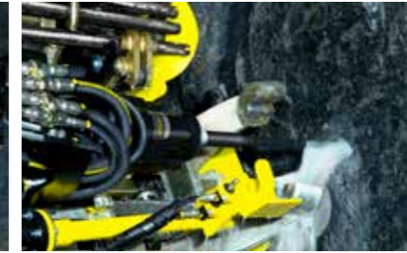
The COP RR11 rock drill is optimized for bolt hole drilling. For larger hole diameters required for some friction bolt types the optional COP RR14 is suitable.
