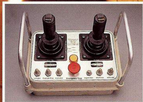
The Halman EN Creter remote unit controls all boom, stabilizer and spray head functions.
