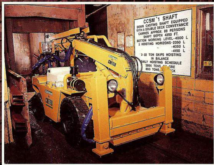
Pictured above, The Halman EN Creter exits a 5 by 14 foot man-cage at INCO Limited's Copper Cliff South Mine.
