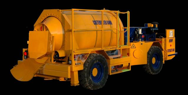
Standard 3.7 m³ (4.8 yds³) drum capacity
