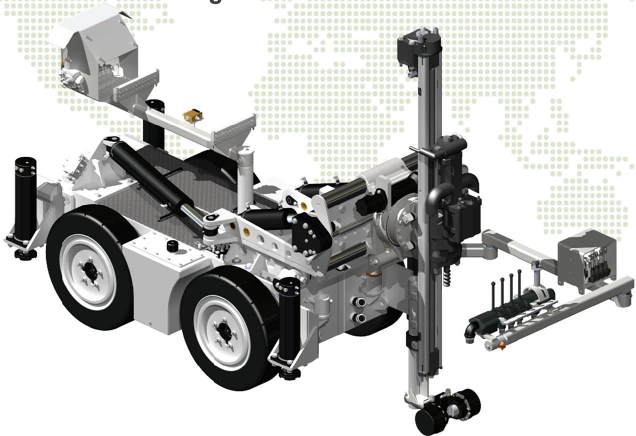
The CMAC PLH is a pneumatic/hydraulic drilling rig for production long-hole drilling and ground support applications for underground mining. The CMAC PLH is a popular pneumatic drill used for long-hole drilling in narrow-vein underground operations.
