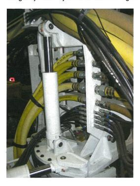
Figure 3-12: Traverse Dump Actuator
