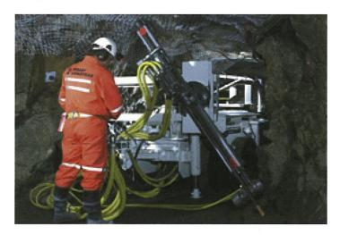
Figure 4-11: Feed Positioning
