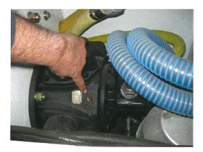
Figure 5-17: Main Air Motor Fill Point
