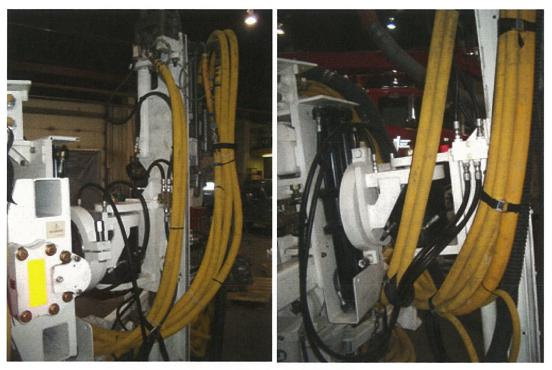
Figure 3-10: Feed Rotation/Swing Unit
