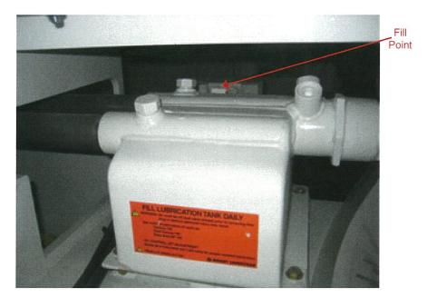
Figure 4-6: Lubricator Fill Point
