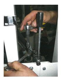
Figure 5-7: V5 Pressure Adjustment
