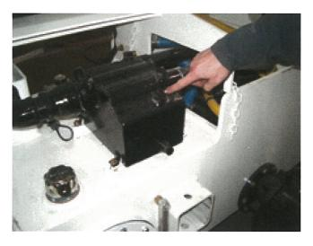
Figure 3-14: Rockdrill Lubricator Fill Point
