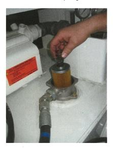
Figure 5-13: Remove Filter Element
