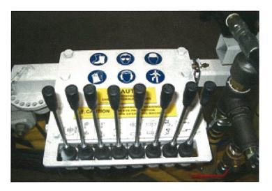
Figure 5-3: V2 Control Valve Bank
