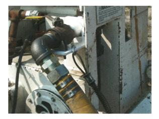
Figure 4-8: Main Air Shut Off Valve
