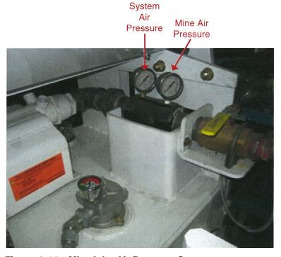
Figure 4-10: Mine Inlet Air Pressure Gauge
