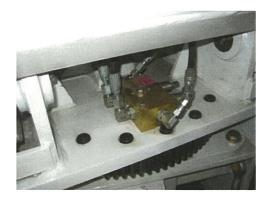
Figure 5-9: V10 Dual Counterbalance Valve
