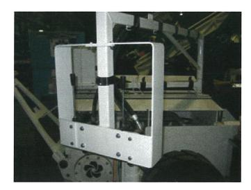
Figure 4-1: Tramming Controls
