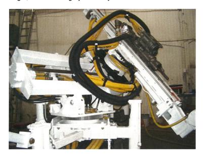
Figure 3-9: Feed Traverse Positioning System
