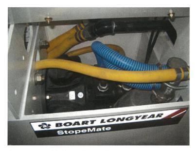
Figure 3-13: Air Motor/Hydraulic Pump
