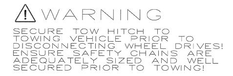
Figure 1-4: Warning Decal: Towing
