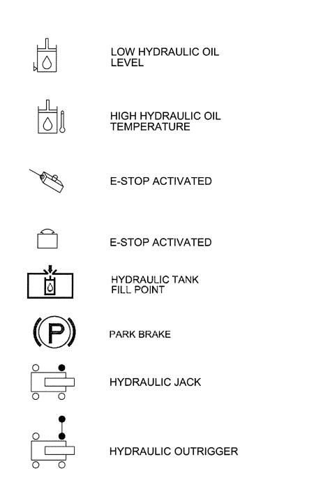
Figure 3-5: Decals Used on the Rig
