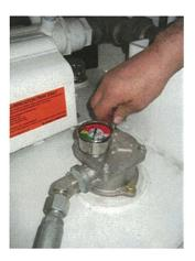
Figure 5-12: Remove Return Filter Cover
