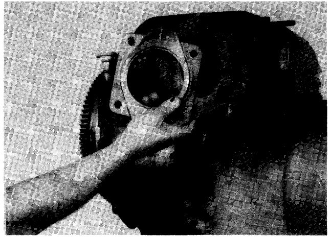
Figure 8 Remove pump adaptor bolts, adaptor and gasket.
