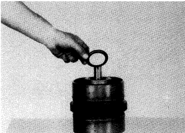
Figure 183 Remove retainer ring retaining washer.
