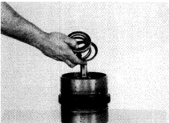
Figure 184 Remove return spring retainers and spring.
